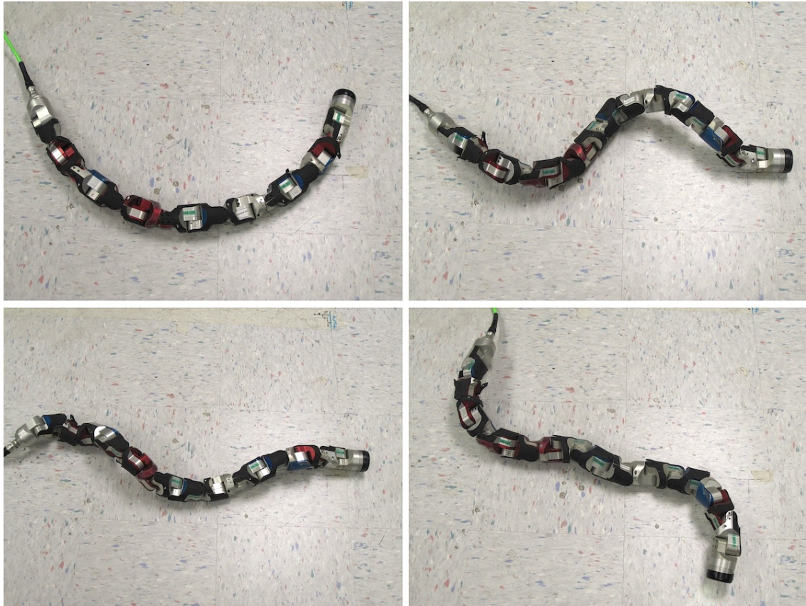
Figure 1: Examples of a snake robot executing the gaits discussed in this paper. Moving across from top left to bottom right: rolling, sidewinding, slithering, and turn-in-place.
