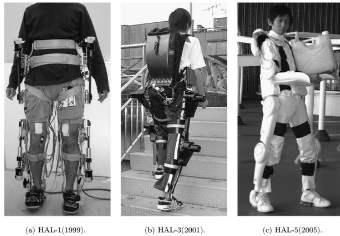
Figure 2.6: Hybrid Assistive Limb - HAL. HAL-1 and HAL-3 support the legs and HAL-5 the legs and the arms. [38].
