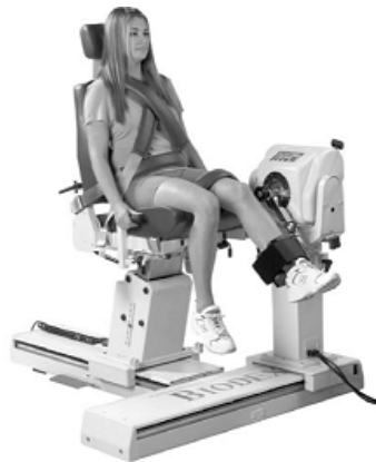
Figure 2.11: Biodex System 3 Isokinetic Dynamometer. In this figure, the Biodex system is used for knee extension/flexion. Different modes of operation like isokinetic, passive, isometric (concentric and eccentric), isotonic and reactive eccentric mode for various joints are supported [5].
