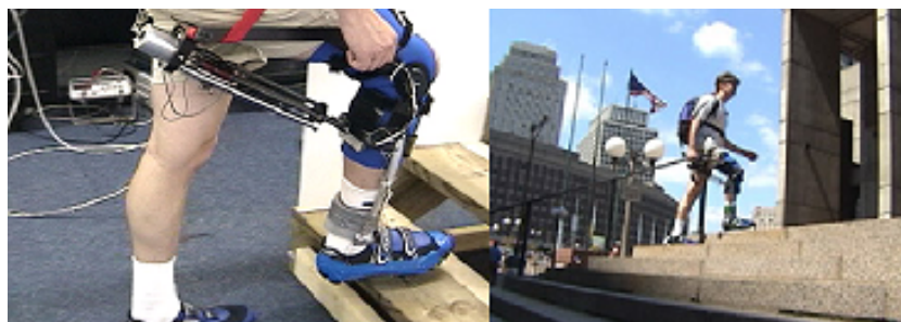
Figure 2.4: Active knee walking orthosis (RoboKnee). The batteries in the backpack allow heavy usage up to 60 minutes [8].
