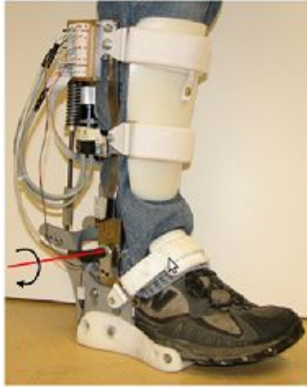
Figure 2.17: Powered ankle foot orthosis. The arrow indicates the degree of freedom of the device. It uses a Robotic Tendon to generate a torque about the ankle [14].
