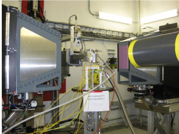
Fig. 11: VULCAN beamline of the Oak Ridge National Laboratory. The setup was rotated 45 deg away from the incoming beam.
