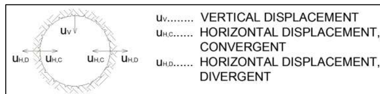
Fig. 63: Convergent and divergent deformation behavior
