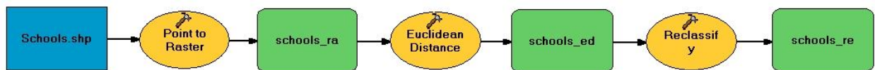
Figure 10: First workflow segment from the raster conversion, to the Euclidean distance calculation, and finally to the reclassify process
