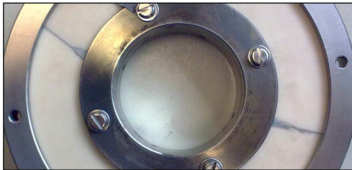
Figure 14: Bonded crack formations of the ceramic ring
