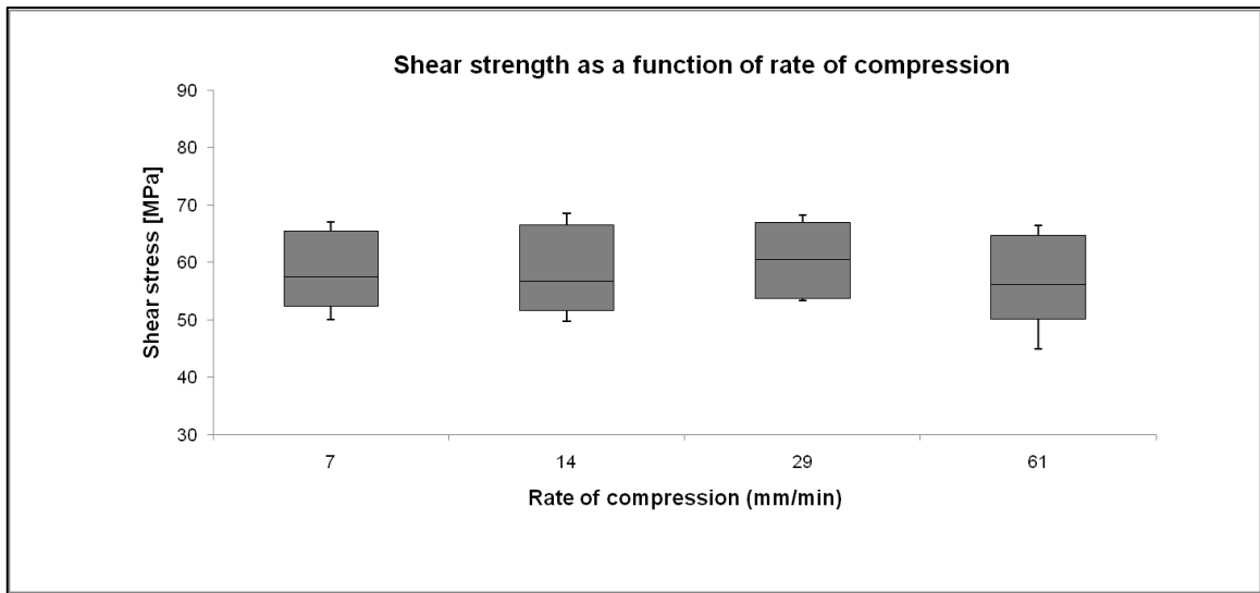
Figure 43: Shear strength as a function of the rate of compression; (conditioning time: 120s, compression time: 180s)
