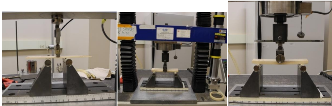
Figure 20: Bending test set up for individual VTC veneer samples (left) and for the 5 layers laminates (middle and right)
