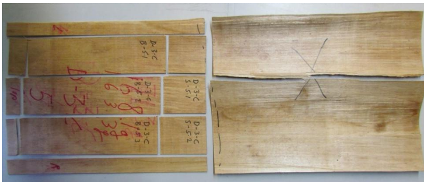
Figure 12 Sizing of VTC samples for bending and shear block test
