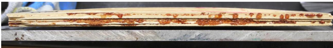
Figure 17 Blows in the middle of the laminate due trapped moisture
