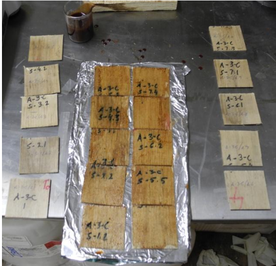
Figure 15 Applied adhesive after allocation
