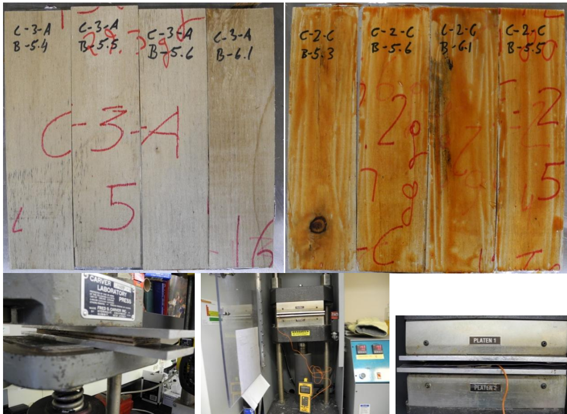
Figure 16 VTC- laminates layup and gluing; Layup (top left); Layup- adhesive applied (top right); pre-pressing (bottom left); pressing with temperature control (bottom middle); press platen in press position with thermocouple wire (bottom right)
