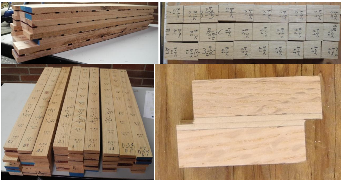
Figure 19 Shear test samples glued on oak substrates after pressing (left) and after cutting (right)
