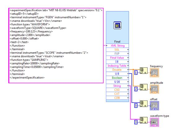
Figure 12: Extraction of parameters from configurable xml parser express VI.
