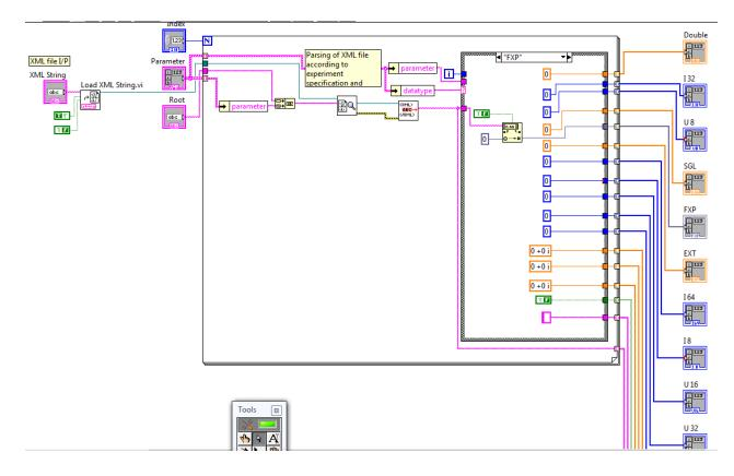
Figure 10: Block diagram of the final source VI ; final.vi Block Diagram
