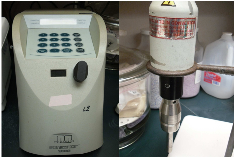
fig. 1: High intensity ultrasonic device „Sonicator 3000“ of Misonix (Perchermeier, 2010)
