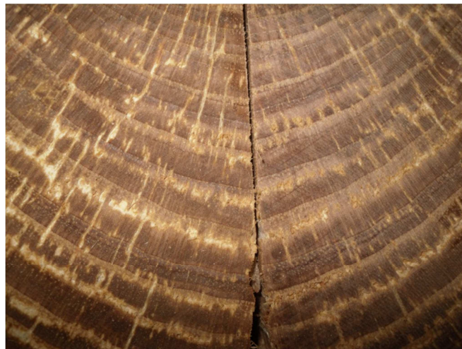
fig. 3: fresh cut Hickory infected with fungi (Perchermeier, 2010)
