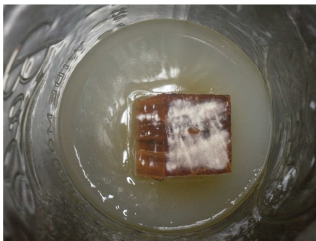
fig. 12: Hickory sample, 3 days after ultrasonic treatment (Perchermeier, 2010)
