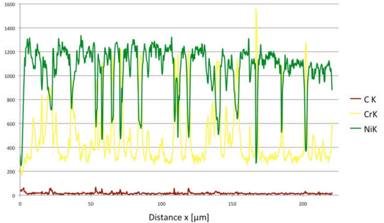
Graph 5: The chromium-carbides are clearly visible due to the drastic decrease of nickel and the chromium spikes.
