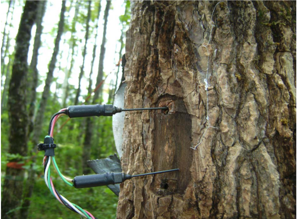
Figure 4 Thermal dissipation probes used to determine sap flow at the Oak Ridge FACE experiment. The probes were normally covered with Styrofoam and got just pulled out from the stem. A callus around the whole formed only during this growing season can be seen.
