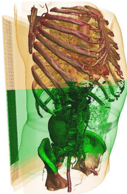
Figure 6.1: Mixed-resolution volume rendering of a large medical dataset. High-resolution bricks are colored in green.
