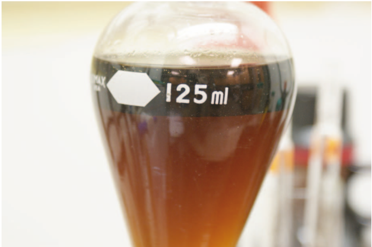
Figure 4: test separation with MIBK
