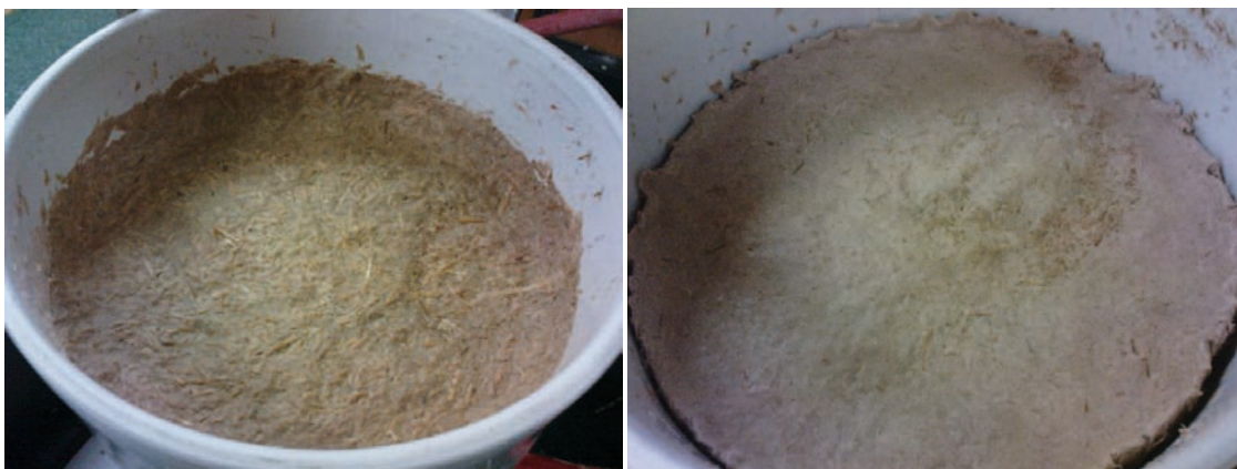
Figure 6: very fibrous material on the left pic (120°C / 0.025 M acid) and ++ breakdown on the right picture (140°C / 0.1 M acid)
