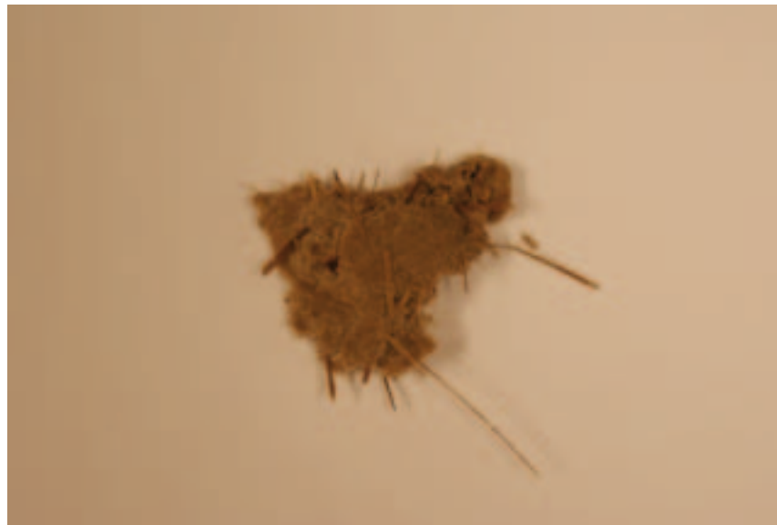
Figure 7: cellulose of a 160 °C run with 0.1 M acid
